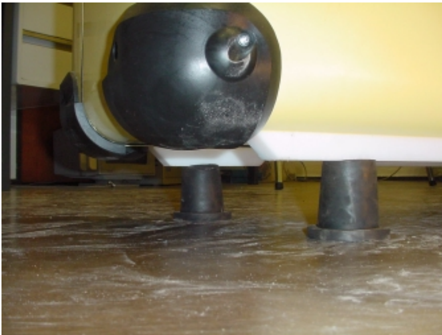
figure 7: The case is during the tests supported on four rubbers
